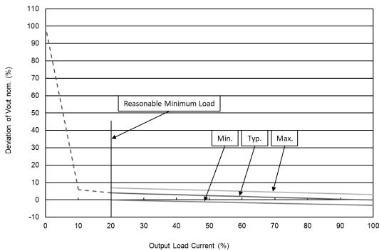
MBU112, MBU113, MBU122 Output Voltage VS Output Load Current
