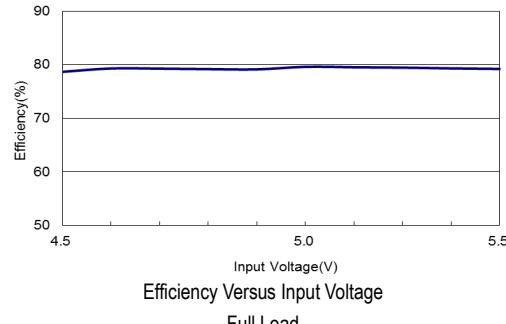
Efficiency Versus Input Voltage
