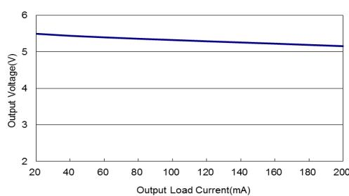
Output Voltage Versus Output Current
