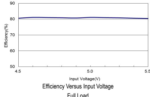
Efficiency Versus Input Voltage
