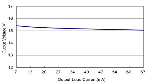
Output Voltage Versus Output Current
