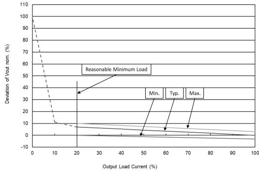
MBU102 &amp; MBU121 Output Voltage VS Output Load Current
