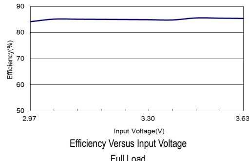
Efficiency Versus Input Voltage
