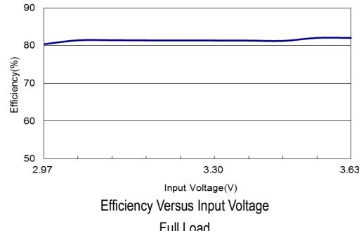
Efficiency Versus Input Voltage
