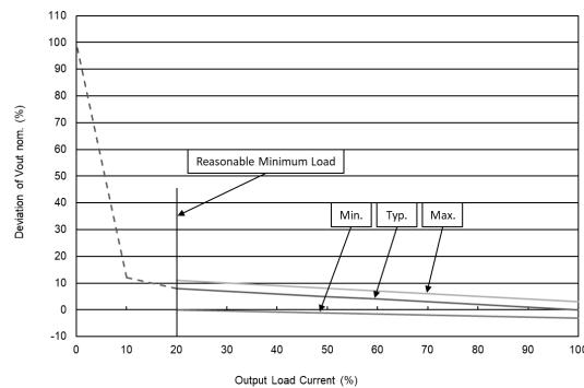
MBU111 Output Voltage VS Output Load Current
