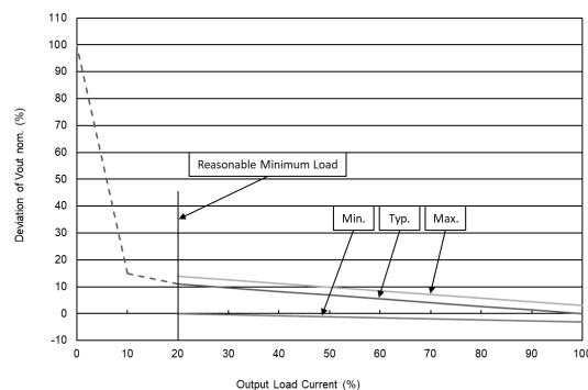
MBU135 &amp; MBU131 Output Voltage VS Output Load Current
