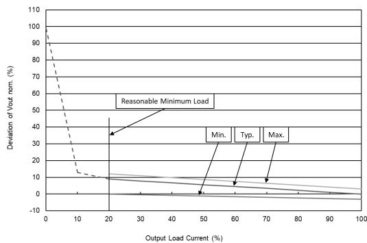
MBU105 &amp; MBU101 Output Voltage VS Output Load Current
