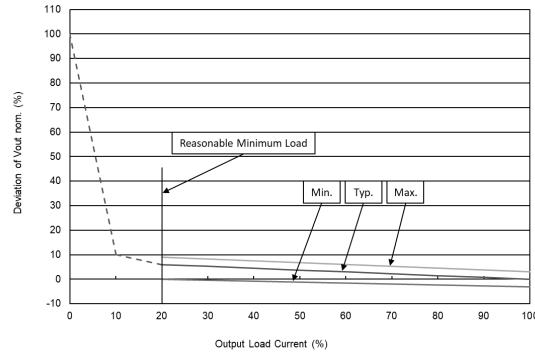
MBU103 Output Voltage VS Output Load Current
