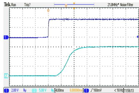
ON/OFF Voltage Start-Up and Output Rise Characteristic
