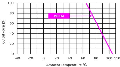
Derating Output Current Versus Ambient Temperature
