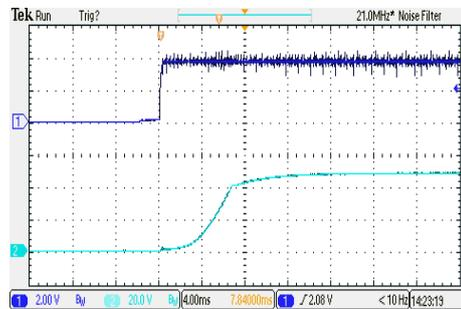
ON/OFF Voltage Start-Up and Output Rise Characteristic
