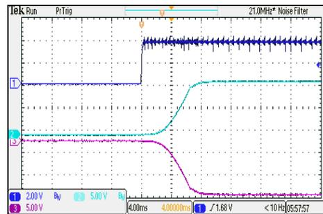
ON/OFF Voltage Start-Up and Output Rise Characteristic
