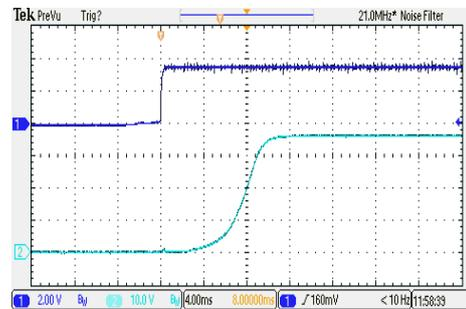
ON/OFF Voltage Start-Up and Output Rise Characteristic
