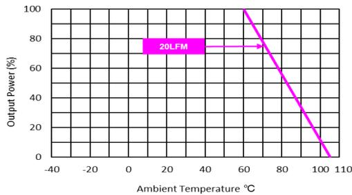
Derating Output Current Versus Ambient Temperature
