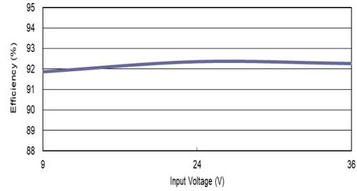
Efficiency Versus Input Voltage
