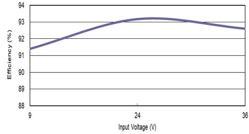
Efficiency Versus Input Voltage
