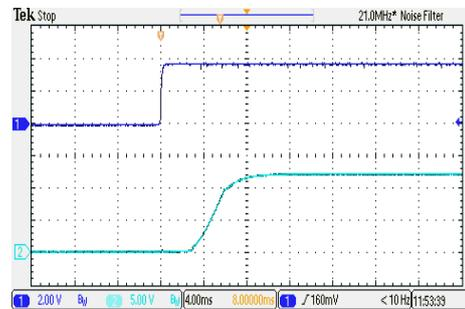
ON/OFF Voltage Start-Up and Output Rise Characteristic
