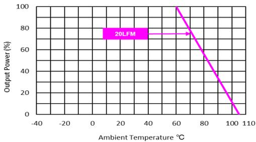
Derating Output Current Versus Ambient Temperature
