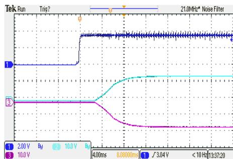
ON/OFF Voltage Start-Up and Output Rise Characteristic
