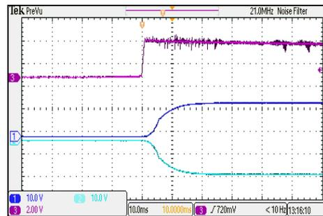
ON/OFF Voltage Start-Up and Output Rise Characteristic
