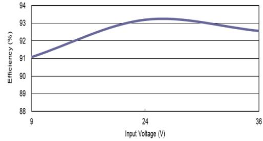
Efficiency Versus Input Voltage
