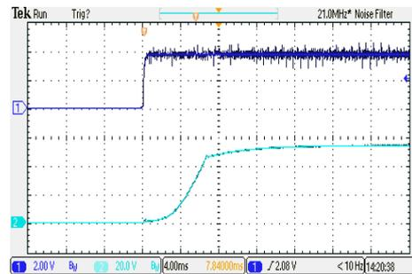
ON/OFF Voltage Start-Up and Output Rise Characteristic
