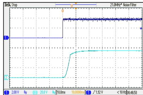
ON/OFF Voltage Start-Up and Output Rise Characteristic
