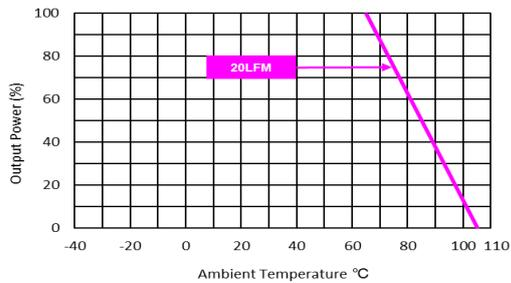
Derating Output Current Versus Ambient Temperature
