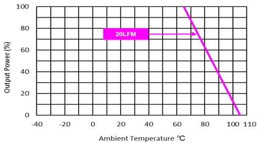
Derating Output Current Versus Ambient Temperature
