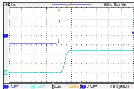
ON/OFF Voltage Start-Up and Output Rise Characteristic
