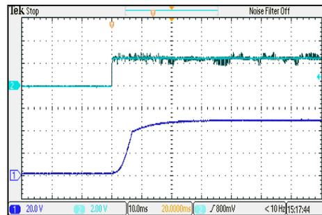
ON/OFF Voltage Start-Up and Output Rise Characteristic
