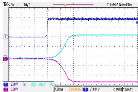
ON/OFF Voltage Start-Up and Output Rise Characteristic
