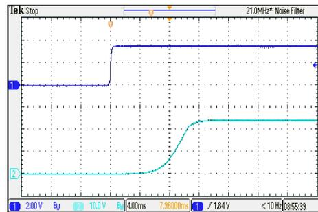
ON/OFF Voltage Start-Up and Output Rise Characteristic
