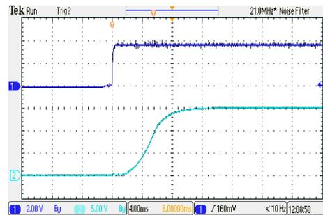
ON/OFF Voltage Start-Up and Output Rise Characteristic
