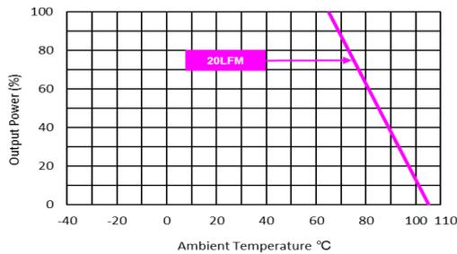
Derating Output Current Versus Ambient Temperature
