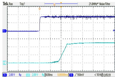
ON/OFF Voltage Start-Up and Output Rise Characteristic
