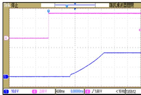
ON/OFF Voltage Start-Up and Output Rise Characteristic
