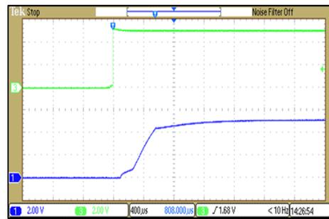
ON/OFF Voltage Start-Up and Output Rise Characteristic
