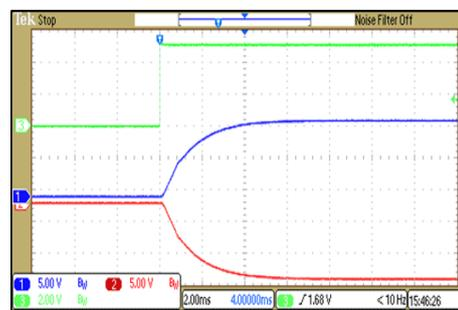
ON/OFF Voltage Start-Up and Output Rise Characteristic
