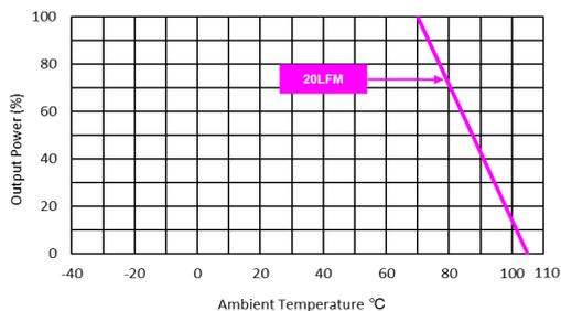
Derating Output Power Versus Ambient Temperature
