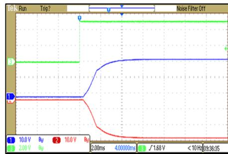
ON/OFF Voltage Start-Up and Output Rise Characteristic
