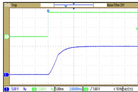
ON/OFF Voltage Start-Up and Output Rise Characteristic
