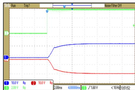
ON/OFF Voltage Start-Up and Output Rise Characteristic
