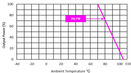
Derating Output Power Versus Ambient Temperature
