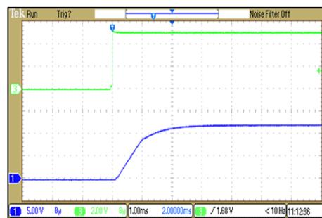
ON/OFF Voltage Start-Up and Output Rise Characteristic
