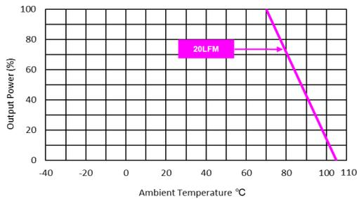
Derating Output Power Versus Ambient Temperature
