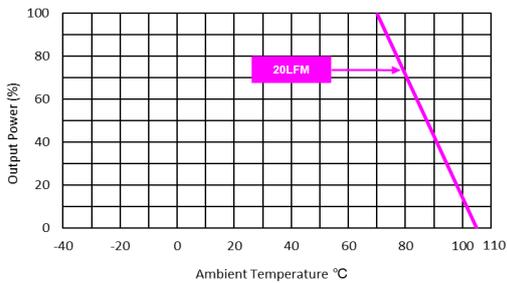
Derating Output Power Versus Ambient Temperature
