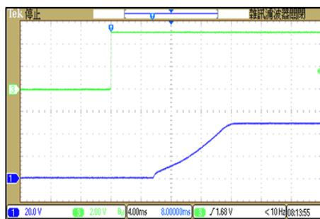
ON/OFF Voltage Start-Up and Output Rise Characteristic
