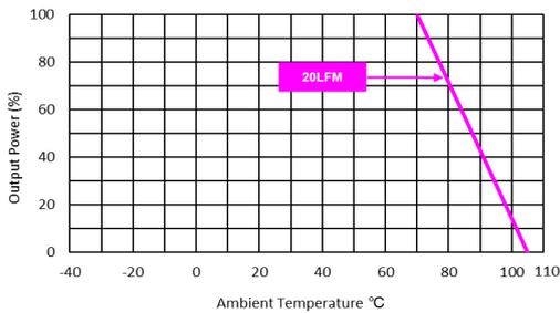
Derating Output Power Versus Ambient Temperature
