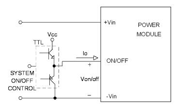
Level Control Using TTL Output
