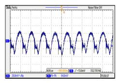
Typical Output Ripple and Noise  $V_{\text{in}}\text{=}V_{\text{in nom}}\,;\,\text{Full Load}$
