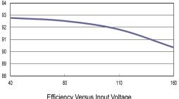
Efficiency Versus Input Voltage Full Load
