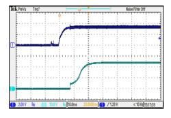
Typical Input Start-Up and Output Rise Characteristic  $V_{\text{in=}} \! = \! V_{\text{in nom}} \; ; \; \text{Full Load} \;$
