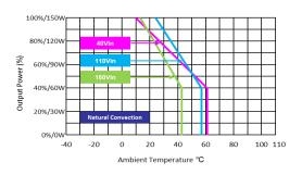
Derating Output Power Versus Ambient Temperature (with HS7 heatsink)
