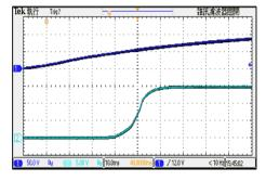
Typical Input Start-Up and Output Rise Characteristic  $V_{\text{in=}} \! = \! V_{\text{in nom}} \; ; \; \text{Full Load} \;$
