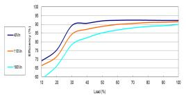
Efficiency Versus Output Current
