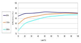
Efficiency Versus Output Current
