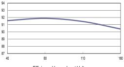
Efficiency Versus Input Voltage Full Load
