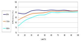
Efficiency Versus Output Current
