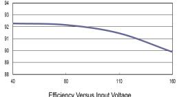
Efficiency Versus Input Voltage Full Load
