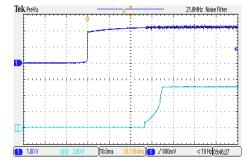
ON/OFF Voltage Start-Up and Output Rise Characteristic  $V_{\text{in=}} \! = \! V_{\text{in nom}} \; ; Full \; Load$
