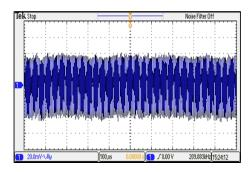
Typical Output Ripple and Noise  $V_{\text{in}}\text{=}V_{\text{in nom}}\,;\,\text{Full Load}$
