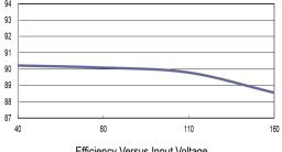
Efficiency Versus Input Voltage Full Load
