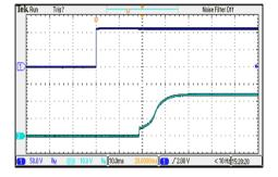
ON/OFF Voltage Start-Up and Output Rise Characteristic  $V_{\text{in=}} \! = \! V_{\text{in nom}} \; ; Full \; Load$
