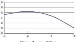
Efficiency Versus Input Voltage Full Load
