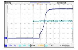
ON/OFF Voltage Start-Up and Output Rise Characteristic  $V_{in=}=V_{in nom}$ ; Full Load
