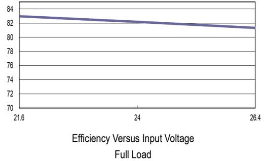
Efficiency Versus Input Voltage Full Load
