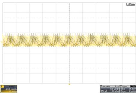
Typical Output Ripple and Noise
