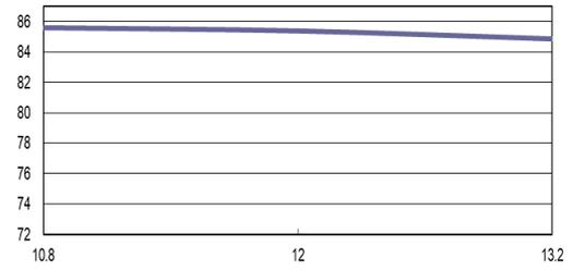
Efficiency Versus Input Voltage
