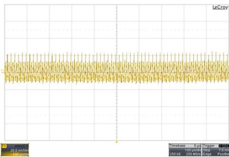
Typical Output Ripple and Noise
