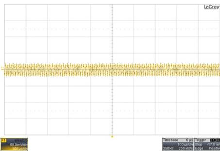
Typical Output Ripple and Noise
