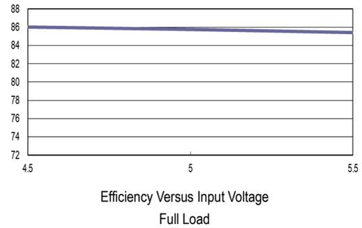
Efficiency Versus Input Voltage Full Load
