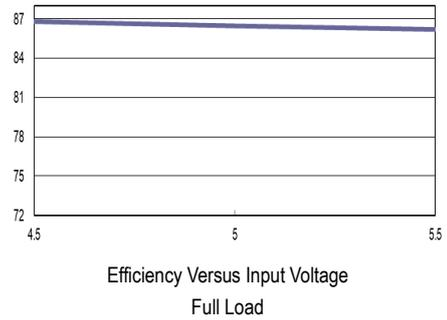
Efficiency Versus Input Voltage
